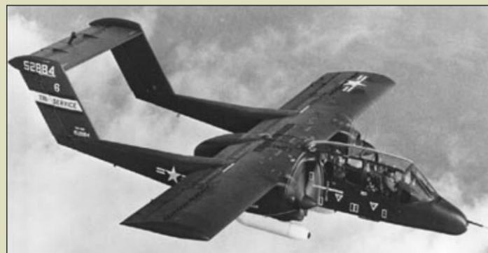
**LEFT One of seven prototype Broncos, YOY-10A BuNo 152884; the first of them flew on July 16, 1965, at Columbus, Ohio. Production aircraft had greater wingspan and more widely-spaced booms.**
